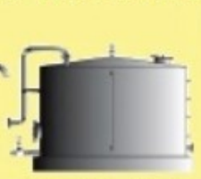
Coned Roof Tank
